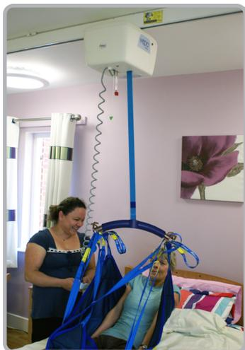
The hand control features light touch pneumatic buttons creating a safe operating system, ideal for bathing, and incorporates colour coded buttons which correspond to coloured arrows on the hoist to give clear indication of the direction of travel.
