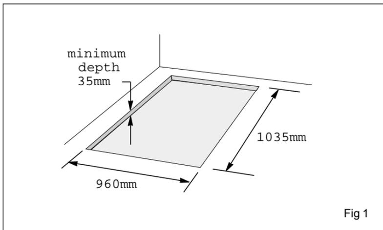
2. Ensure the floor is flat before fitting the shower cubicle base into it (use leveling compound or a dry mix).
